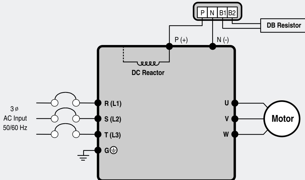
For 37~90kW (50~125HP) Built-in DCL Type
