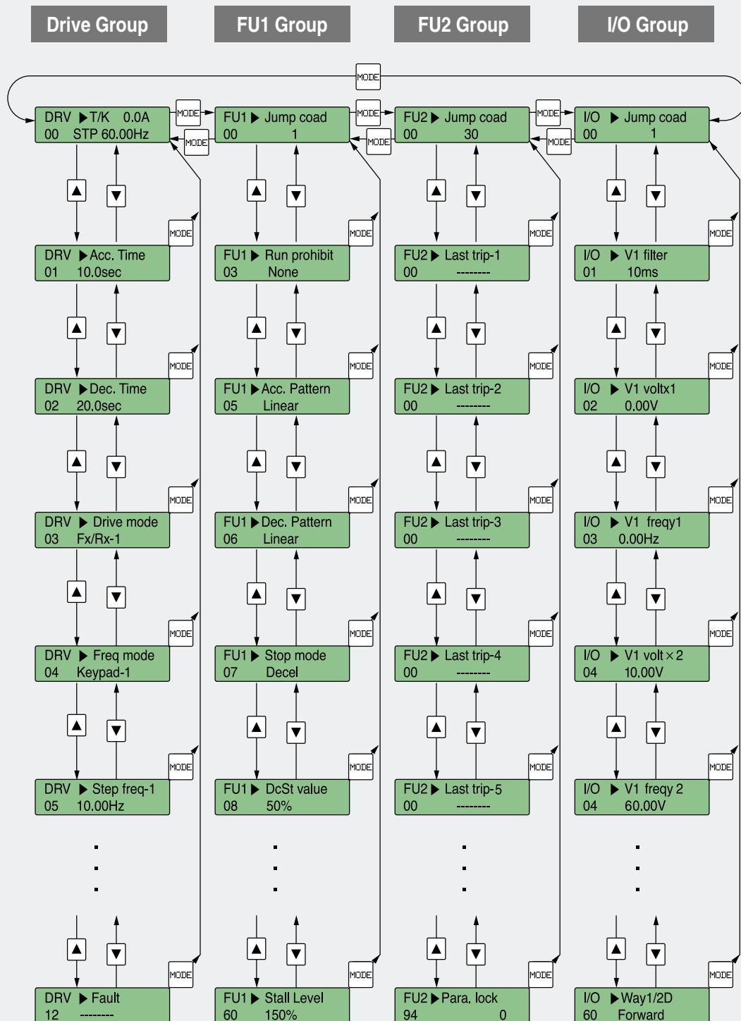
(Note) This figure shows group and code navigation through LCD display keypad. It can be different from actual display due to the group addition or code change.
