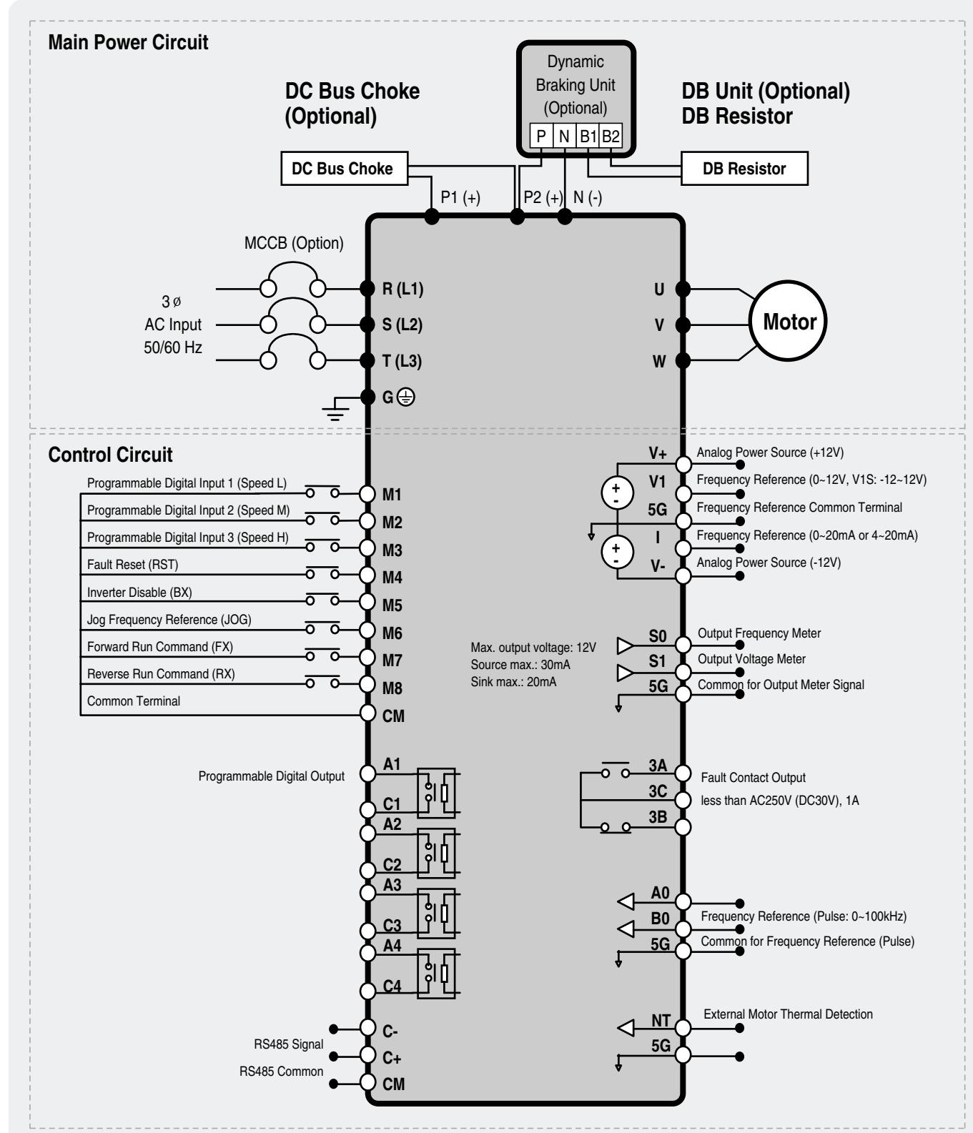
Note 1) 5G is Common Ground for Analog Input / Output.
