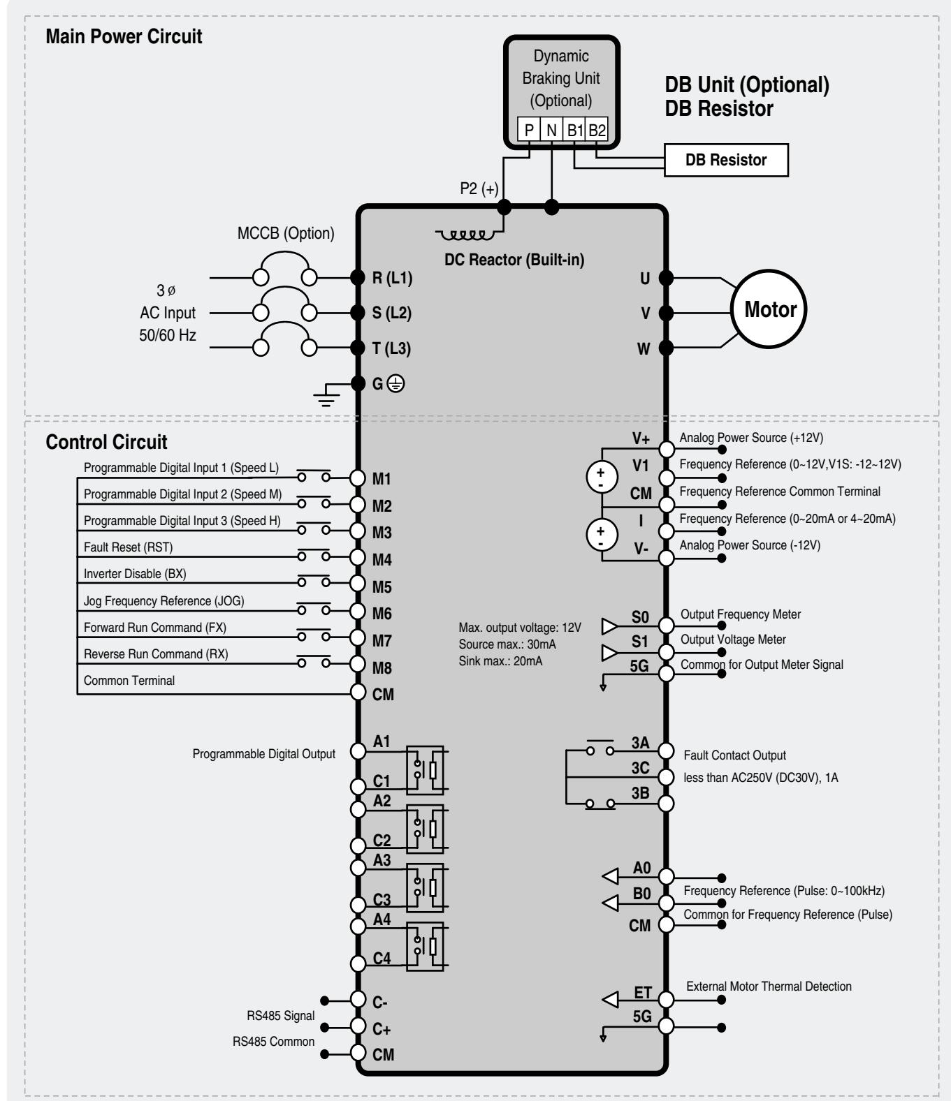
Note 1) 5G is Common Ground for Analog Meter Output (S0, S1) and External motor thermal detection (ET).
