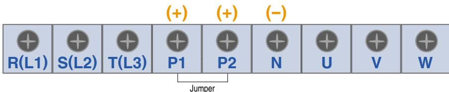
● 15~18.5kW (20~25HP) <Built-in DC Reactor Type, 400V Class>
